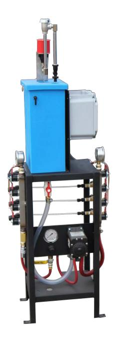
The TMXSF Presoak Tire/Motor Clean system is a foaming presoak or tire/motor clean system that will deliver foaming product to multiple bays. Constructed with a stainless steel manifold and a combination of stainless steel and brass wetted parts to resist corrosion. The air driven double diaphragm pump maintains constant supply volumes and operates on a demand basis by pumping at a higher or lower rate as required.
