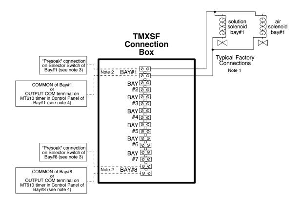
Note 1: These connections are made at the factory. Connections for the other bays that the foam system is equipped to support are also made at the factory in a manner similar to that shown for bay#1.
